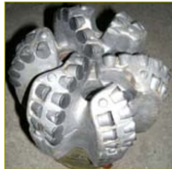
PNEU #2113E (M1666BDP E006) 4890' at 91.4 ft per hr Dull grade 1-3-WT-A-X-1N-NO-TD
