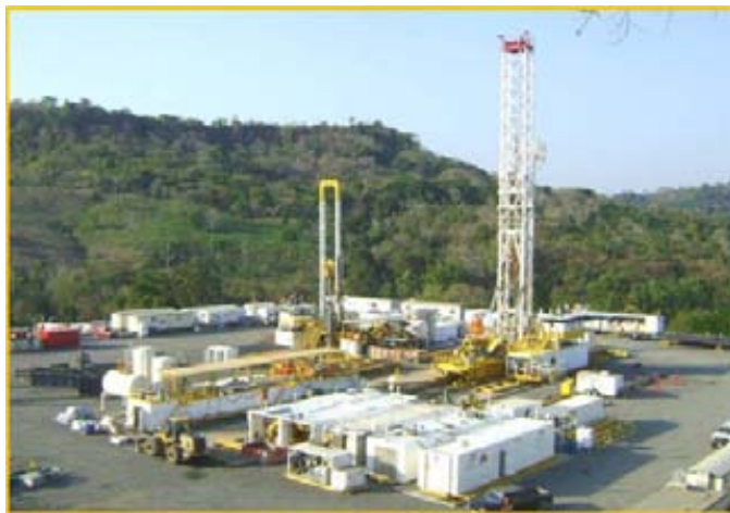
Xtreme Coil's Rig #3, an XTC 200 (left), and Rig #17, an XTC 400, drilling on the same well pad in the Chicontepec project in México.
